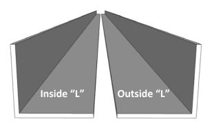
channels spaced approximately 36" apart and secure the channel with screws. The second "L" will be installed after the wall panels are fastened in place.
