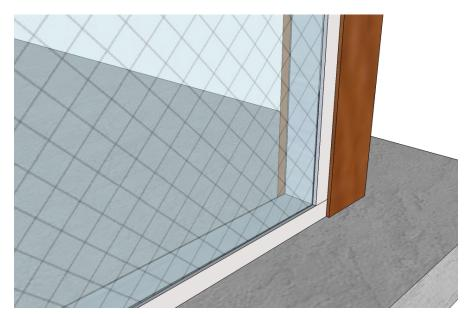
by shimming them at the bottom to the desired height. Make sure that the receiving channels do not cover the screen spline groove. Fasten the panels with Zip screws going through the channel and into the
