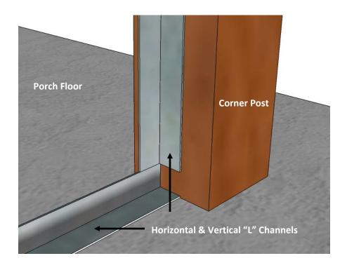
2. Measure the heights of the vertical supports between the horizontal receiving channels and cut the "C" and "L" channels. Install the "C" at one side and the "L" at the other.
